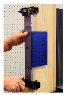
To attach the clamp, just slide over the post and tighten to the door.
