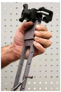
Thread the pointer in the center hole of the five tapped holes as shown.
