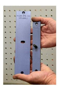
Shown is the HIT-45ML1 alignment fixture. This is used to align the function holes used by the mortise lock to the correct location in the mortise pocket. It will work with any of our mortise lock templates that use a 1-1/4" wide by a 8" tall faceplate.
