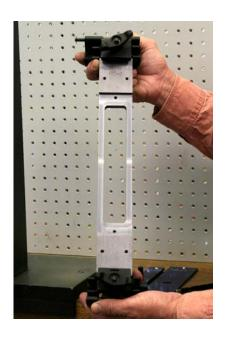
This is the HIT-45 clamp that will be used to install a mortise lock. It can be used to install a variety of hardware using interchangeable templates.
