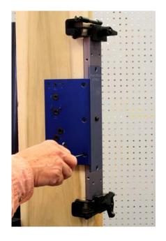
This clamp can be used with one or two templates. If using only one template prep one side of the door and with the clamp still in position, remove the template and install on the other side.
