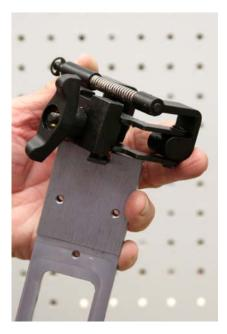
The clamp heads will now spin left to right. This will allow the clamp to align to the door bevel.
