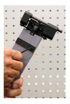
Attach the bevel blocks both top and bottom on the inside of the HIT-45 clamp with the supplied 10-32 x 1/2" flat head socket screws. These blocks pick up the door bevel.
