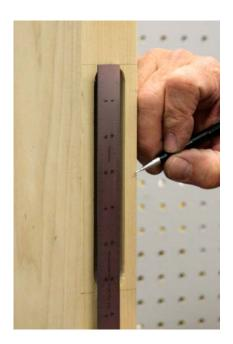
Measure the distance between the top and bottom of the mortise and divide by two.
