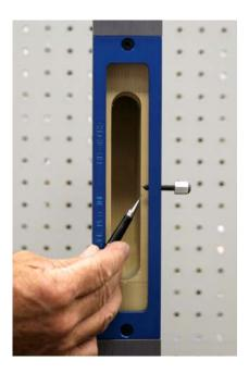
Hold the HIT-45 to the door with the locating pointer pointing to the center line, allow the bevel blocks to conform the door bevel and tighten clamps. Double check the pointer is located to center and remove the pointer.
