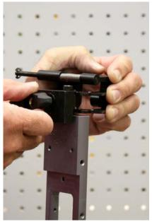
Loosen the black plastic knob until you can rotate the vise block 180 degrees, this will allow it to rotate freely. Repeat this procedure with the other end of the clamp.
