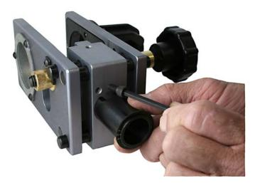
There are three drill guides supplied with the HIT-50 for use when drilling the edge bore, they are held in with a allen screw. Choose from a 7/8", 1" or the brass guide for use with a multi-spur bit.
