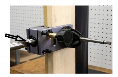
When drilling through the door, use a slower speed and be sure to back out the drill several times, this will allow the wood chips to be cleared from the work. This will provide a cleaner cut and a cooler running bit.
