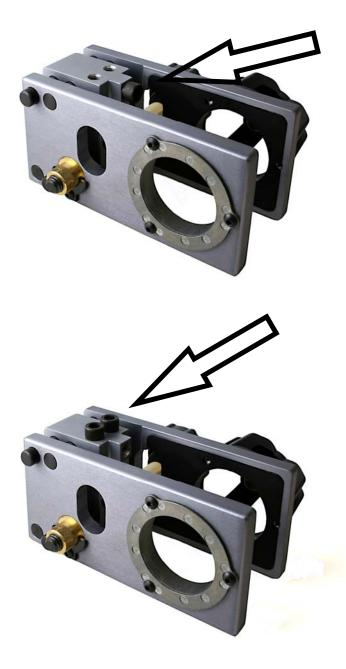
To adjust for 2-3/8" backset locks, install the backset studs as shown in picture. Make sure studs are fully threaded in.
