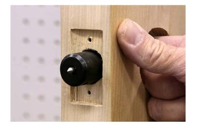
Don't forget to mark the jamb for the strike plate. Shown is our HIT-44SL8 1" strike locator.
