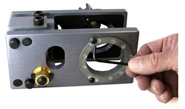
Using the supplied allen wrench, install the proper size break out plate/hole saw guide. Two 1-1/2" and two 2-1/8" guides are supplied. For steel door use, remove the multi-spur guide on opposite side and replace with another guide as shown in picture.
