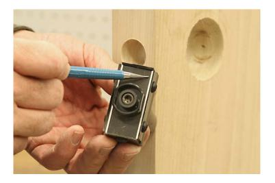
Here we are using our HIT-44LM3 latch marking tool to mark the area for the faceplate. There is a 1/16" shim that is used to adjust to a 1" or 1-1/8" face. With the shims on the inside, this will mark a 1-1/8" face.
