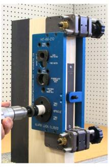
Change to a 1-1/4" hole saw and drill the lever hole. This hole goes to the mortise pocket from both sides of the door.
