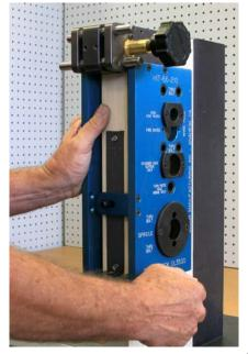
Slide the HIT-66 alignment fixture over the alignment pin and tighten to door. Alternate tightening between the top and bottom clamp. Do not attempt to tighten one clamp all the way at once.
