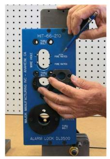
There are two positions for the wire hole. One for fire rated doors and the other for non-fire rated. Choose the location and install the 3/4" diameter drill guide.
