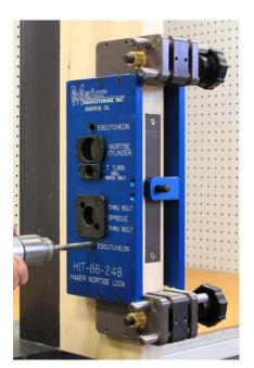
With the 3/8" bit still in the drill, drill the top and bottom escutcheon trim holes. Drill these from both sides of the drill guide.
