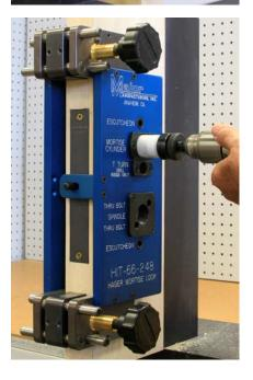
Use a 1-1/4" hole saw to drill the mortise cylinder hole on the outside of the door. Again, back the hole saw out a few times to clear saw dust from the cut.
