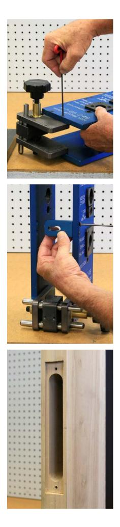
With both clamps opened equally, install both inside and outside templates to the HIT-66 clamp as shown. Do not tighten the 10-32 screws at this time. When all screws have been loosely installed, then it is ok to tighten.
