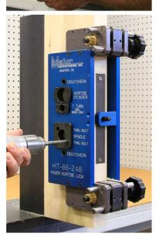
With a 3/8" twist drill, drill the thru bolt holes on both sides of the door. These holes go to the mortise cavity. Do not attempt to drill from one side through to the other.
