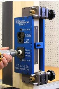
Use a 1" hole saw to drill the spindle hole. Drill this hole to the mortise pocket from both sides of the door. When drilling back the hole saw out a few times to clear saw dust from the cut.
