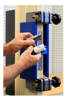
Use a 1-1/4" hole saw and drill for the mortise cylinder. A standard hole saw will work on wood or steel door. Our HIT-48-114 carbide tip hole saw can also be used on wood doors only.
