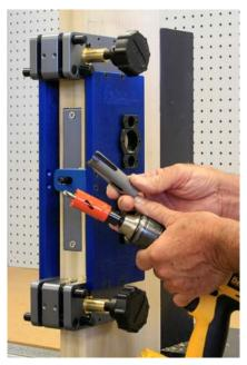
Drill the 1" hole used for the lock spindle with a hole saw.
