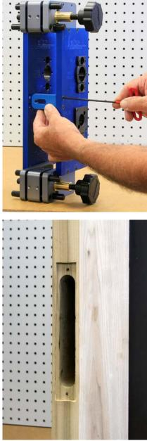
With both clamps opened equally, install both inside and outside templates to the HIT-66 clamp as shown. Do not tighten the 10-32 screws at this time. When all screws have been loosely installed, then it is ok to tighten.
