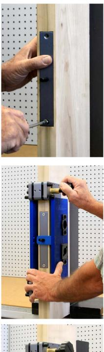
Install the mortise lock positioning plate. The plate will fit into the 1-1/4" x 8" faceplate cut out. There will be a 3/8" diameter pin centered on the plate. There is no top or bottom to worry about.
