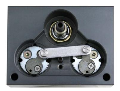
Completed installation of the Schlage Modular cylinders. Link will allow only one key to be removed at a time. Returning one key and turning will allow removal of the other.
