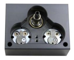
Secure cylinders with two set screws. The cylinder should be flush or a little above the inside of the trap. It may be necessary to run a 8-32 tap down the side of the cylinder / key trap slot for the screw to thread in smoothly.
