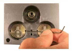
Secure cylinders with two 6-32 set screws. It may be necessary to run a tap down the side of the cylinder prior to installing the the second set screw.
