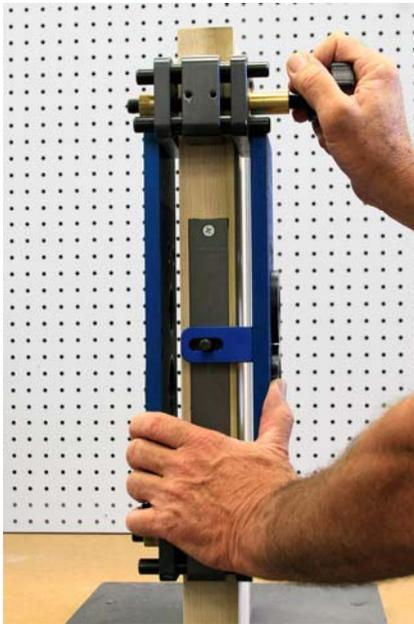
Slide the HIT-66 template with the alignment guide alignment pin and tighten to door. Alternate tightening between the top and bottom clamp. Do not attempt to tighten one clamp all the way at once.
