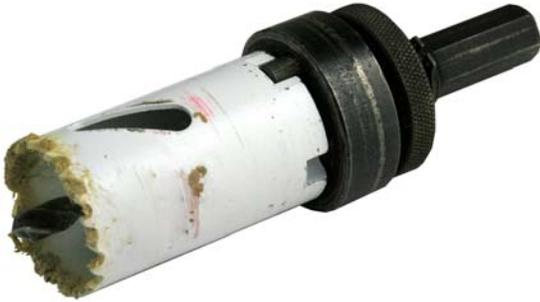
All hole saws are not created equal. A cheap hole saw from a home improvement center or one that has been dropped can be out of round and will not fit the drill bushings in our templates.
