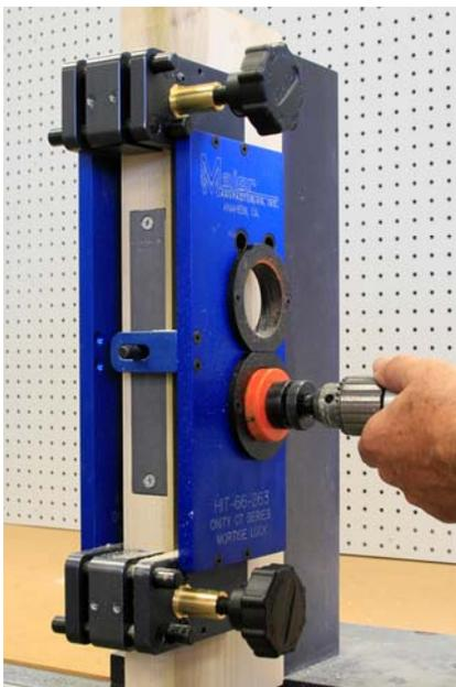
With a good quality hole saw, drill the two 2-1/8" holes to the mortise pocket.
