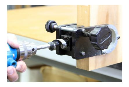
Drill thru to the cross bore in one operation, the screw point on the auger bit will not allow you to pull it out when drilling.
