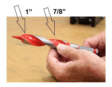
Shown is a 1" DIABLO brand auger bit sold by home centers. While a good bit, it will not work in our drill guide. It is a 1" bit, but the twist is only 7/8" and will not be supported by the guide.
