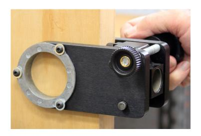
Tighten the main clamp knob. The HIT-49 drill guide will now be securely attached to the door.
