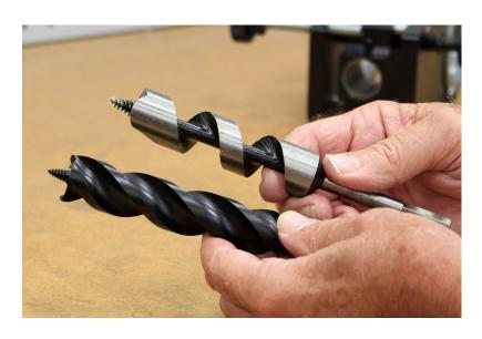
A brad point bit or auger may be used for the latch hole. Here are two examples of auger bits that can be used. Make sure they are a 1" diameter and the twist diameter is also 1" in diameter.
