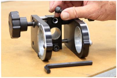
To adjust for 2-3/4" backset locks, remove the two 3/8" cap screws.
