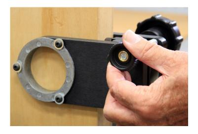
Tighten the cantilever knob, this will prevent the guide from splaying out..
