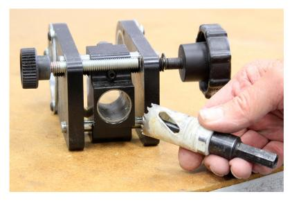
If drilling a steel door, a 1 inch hole saw can be used. NOTE: Because of the way hole saws are made, not all hole saws will fit this drill guide.
