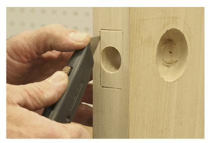
Use a sharp box cutter to deepen the vertical outline left by the marking tool. If you use a chisel for this step you run the risk of splitting out the side of the door.
