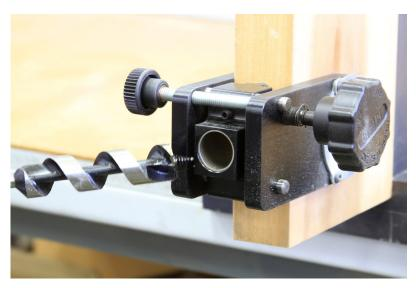
A 1" auger bit being used to drill the latch hole.
