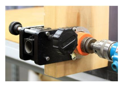
Drill thru from the other side. Use the same procedure of backing out the bit.
