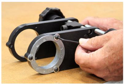
Using the supplied allen wrench, install the proper size hole saw guide. In this case we are using the 2-1/8".
