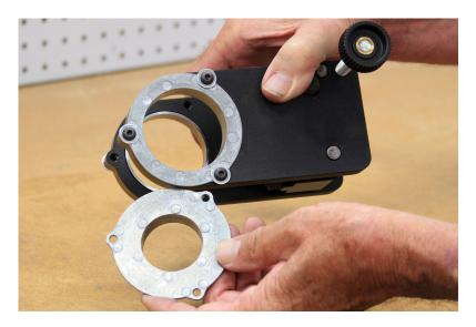
There are two sizes of hole saw guides supplied, 1-1/2" and 2-1/8".
