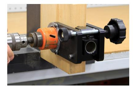
With a hole saw drill half way into the door. Use a lower RPM and back the bit out often to prevent from over heating the bit.
