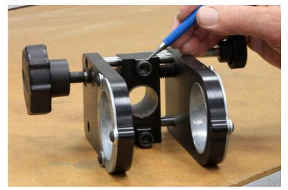
To adjust for 2-3/8" backset locks, install the two 3/8" cap screws as shown in picture. Make sure studs are fully threaded in.
