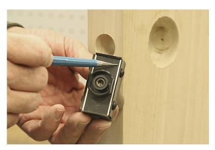
Here we are using our HIT-44LM3 latch marking tool to mark the area for the faceplate. There is a 1/16" shim that is used to adjust to a 1" or 1-1/8" face. With the shims on the inside, this will mark a 1-1/8" face, shims outside will mark a 1" wide faceplate.
